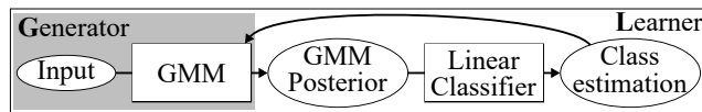
Figure 2. Principal structure of the GMR model, composed of a GMM modeling the distribution of training samples (left). A linear classifier operating on the posterior probabilities (also termed responsibilities ) produced by the GMM. The coupled GMM/classifier implements the Learner, whereas the GMM implements the Generator from Fig. 1. The GMM sampling process is informed by feedback from the classifier.
